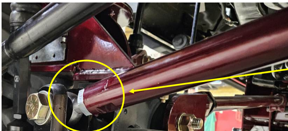
LOWER PAN HARD BAR MOUNT WELDED TO AXLE
