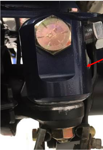
LOWER PANHARD BAR MOUNT AND AXLE GROUND
