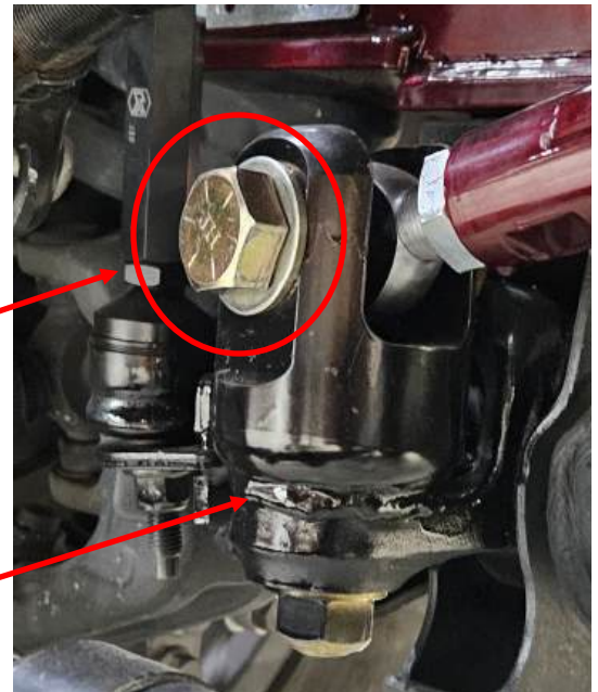
LOWER PANHARD BAR MOUNT AND AXLE GROUND
