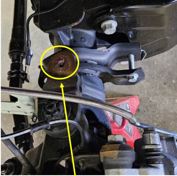
LOWER SPRING MOUNT—INSTALL M14 BOLT HERE
