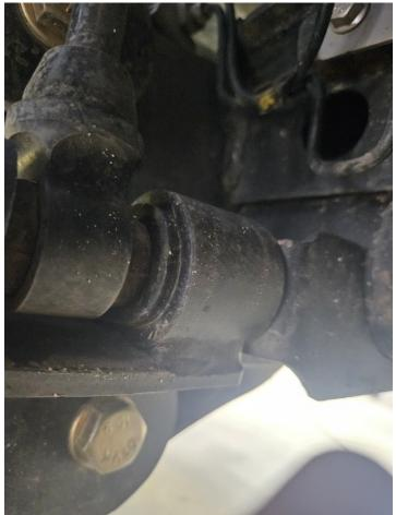
12. LOCATE THE SHOCKS (#10003380). FASTEN THE LOWER END OF THE SHOCK INTO THE SHOCK MOUNT WITH THE 1/2"-20 x 5-1/2" Bolt and slide the round end of the mount in the factory shock location on the axle. Torque this bolt to 125 ft./lbs.
