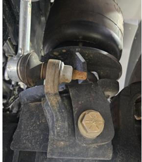
8. FASTEN THE AIR BAGS INTO THE UPPER AIR BAG MOUNTS. USE THE 3/4" AND 1/2" NUTS AND LOCK WASHERS ON THE TOP. TIGHTEN ALL THE NUTS AND BOLTS TO 35 FT./LBS. LOCATE THE AIR FITTING AND INSTALL INTO THE AIR PORT ON TOP OF THE BAG. TIGHTEN FINGER TIGHT AND THEN ONE COMPLETE TURN AFTER THAT.
