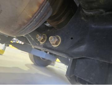
2. LOCATE RADIUS ARM ASSEMBLY (#10034775-DS & #10034756-PS). INSTALL THE RADIUS ARM ASSEMBLY TO THE DROP MOUNT WITH M18-2.5MM X 130MM BOLT. SET THE GAP BETWEEN THE CAST KNUCKLE AND RADIUS ARM TO APPROXIMATELY 2". YOU MAY NEED TO ROTATE THE CAST KNUCKLES TO GET THE CORRECT LENGTH DURING INSTALL. THE RADIUS ARM BOLTS TO THE LOWER FACTORY RADIUS ARM LOCATION WITH THE M18-2.5MM X 130MM BOLTS. TORQUE THE M18 BOLTS TO 150 FT./LBS.
