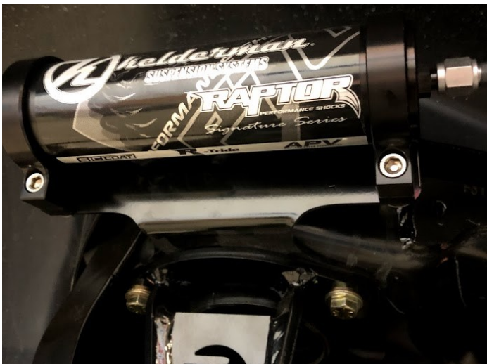
THE REMOTE RESERVOIR SHOCK MOUNT FASTENS IN BETWEEN THE UPPER COIL BUCKET AND UPPER BAG MOUNT
