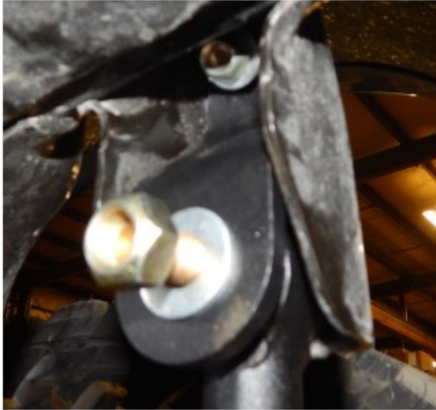
LARGE WASHER ON THE OUTSIDE OF THE BOTTOM END LINK
