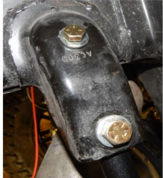
LARGE WASHER ON THE OUTSIDE OF THE BOTTOM END LINK
