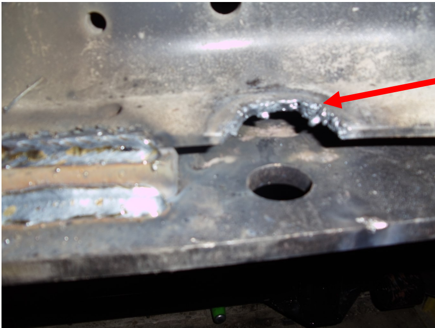
If the factory cross member covers up the air bag hole, use a torch to make clearance.
