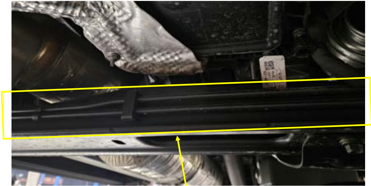
FACTORY DEF LINES THAT NEED TO BE RE-ROUTED
