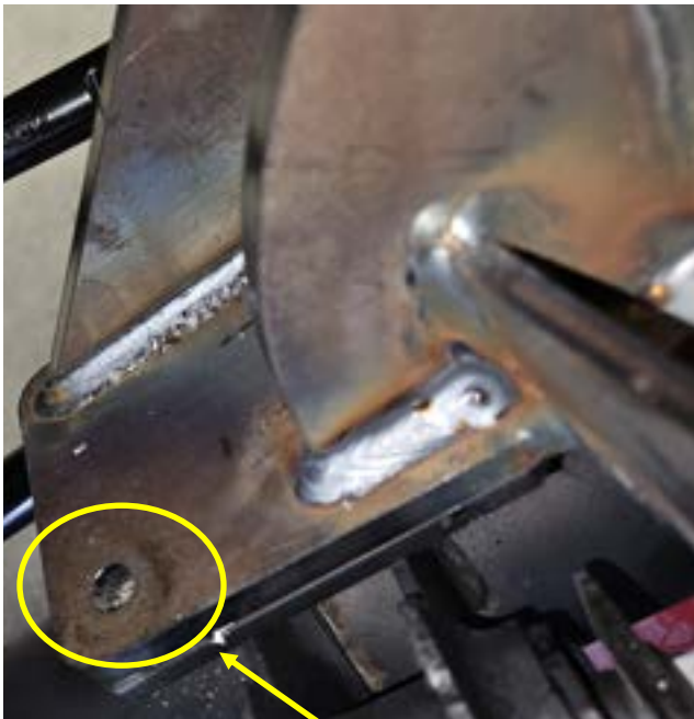
DRILL 17/32" HOLE USING HOLE IN THE PLATE AS A GUIDE
