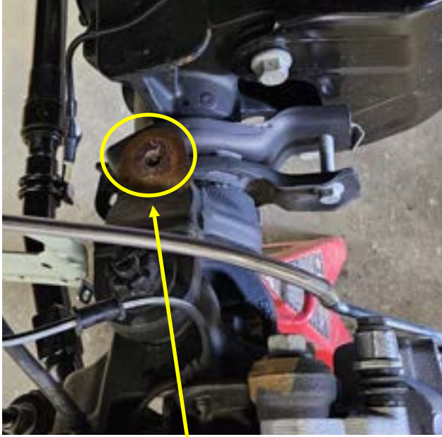
LOWER SPRING MOUNT—INSTALL M14 BOLT HERE
