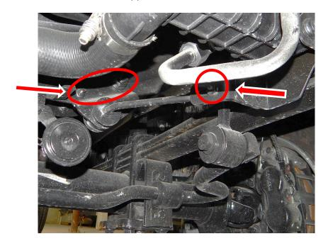
**8**: Remove the sway bar, end links, and end link brackets if equipped.
