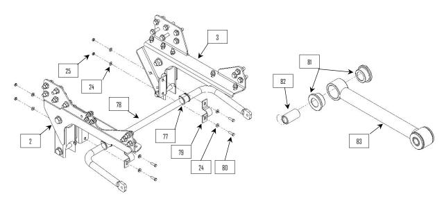
39: Press poly hat bushings (81) and sleeve (82) into both ends of the sway bar end links (83).
