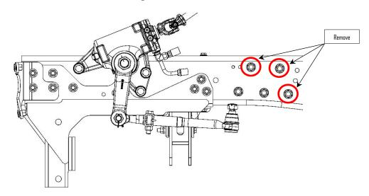
**11:** Align the upper bag plate (21) on the frame using the OEM engine mount bolts. Use 5/8" hardware (4, 7, & 8) to fasten the rear of the of the bag plate to the frame.
