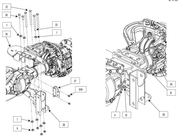
25: Use 1/2" hardware (10, 11, & 39) to fasten the axle clamp (36) to the differential bracket (37).
