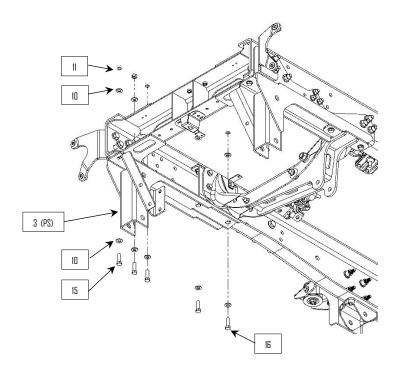
**9**: Check the frame for square using the reference measurements taken in Disassembly *step* 12. Make any required adjustments, once square snug up the installed hardware.
