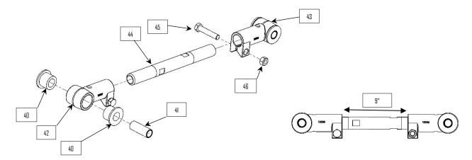
**28**: Use 7/8" hardware (47, 48, 49, & 50) to install the upper trailing arm assemblies into the lower bag plates (30 or 36).
