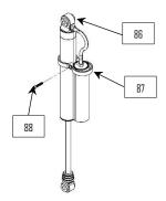
**43**: Use 1/2" hardware (10, 11, & 39) to mount the shocks (86). **NOTE**: Mount the reservoir as high as possible and orient it outward. Check that the reservoir will not contact any steering components or snag any hoses or lines as the suspension & steering travel thru their full sweep.
