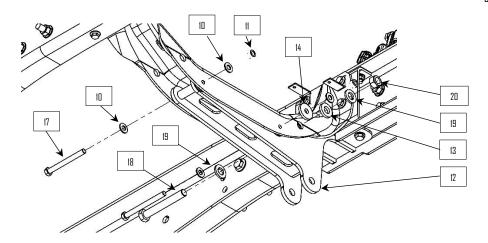
**4:** Install the lower radiator supports removed in Disassembly *step 7*. On the driver's side use spacer washers (13 & 14) to move the core support brace away from the panhard bar crossmember. You will need to Drill the driver's side radiator supports need two holes drilled to 17/32" and 34". The passenger side will need a 17/32" hole drilled.
