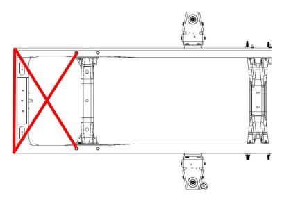
**13**: Remove the shock brackets and the power steering line bracket.
