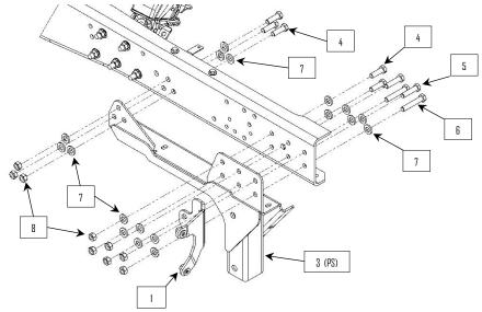
**8:** Fasten the side plate (3) to the bottom frame rail flange using 1/2" hardware (10, 11, 15, & 16).
