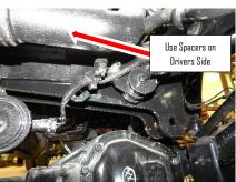
**5**: Fasten the side plate (2) and the panhard bar crossmember (12) to the bottom frame rail flange using 1/2" hardware (10, 11, 15, & 16).
