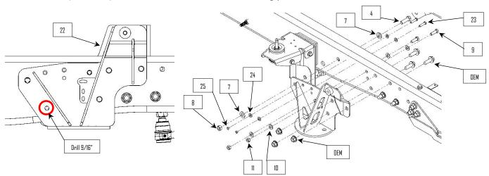
**19**: Use the upper bag plate as a guide to drill a 9/16" hole in the frame rail. Use 1/2" hardware (9, 10, & 11) to fasten to the frame.
