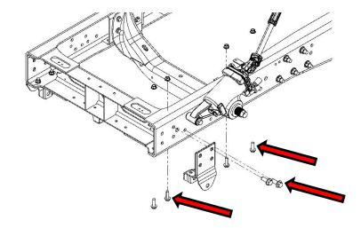
**15**: To remove the huckbolts split the nut using a cutoff wheel or an air chisel.
