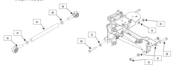
**36**: Install the panhard bar assembly, use 3/4" hardware (19, 20, & 69) **NOTE**: Position grease zerks down. Torque: 3/4"-16 panhard bar bolts should be torqued to 150ft-lb.
