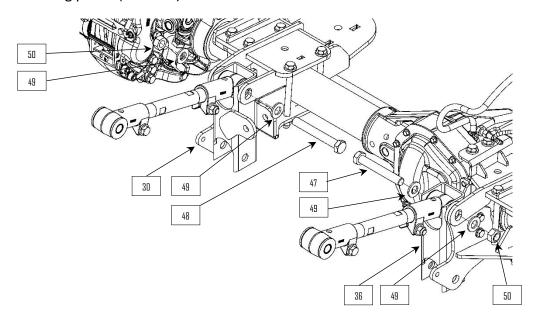
**29**: Once aligned and bolted together tighten down all axle hardware.
