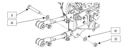
**31**: Bolt the upper and lower trailing arm assembly into the side plate (2 or 3) using 7/8" hardware (49, 50, 51, & 52). **Torque:** 7/8"-14 trailing arm bolts should be torqued to 300ft-lb.
