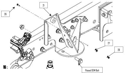
**17**: Use 1/4" hardware (26, 27, & 28) to fasten the power steering lines to the back side of the upper bag plate (21).
