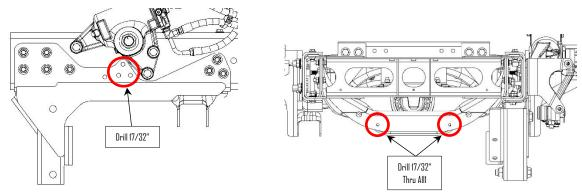
**3**: Bolt the panhard bar crossmember (12) into the second frame crossmember. Use 1/2" hardware (10, 11, & 17) to fasten thru the drilled holes and use 3/4" hardware (18, 19, & 20) in the top hole.
