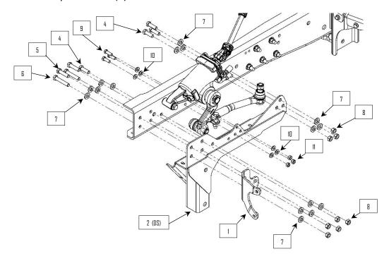
2: Drill out the two smaller holes in the second frame crossmember to 17/32" dia. **NOTE:** On trucks without a factory equipped sway bar. Use the side plate (2) as a jig to drill the three holes located under the steering box.
