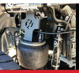
This kit is designed to ride at a height of a 2-3" lift when traveling down the road. However, it is adjustable down to approximately 1" below stock height when deflated and up to an approximate 6" lift when fully inflated. Driving at the maximum height of 6" regularly can stiffen your ride, so we recommend driving at the desired ride height of 2-3" in most driving scenarios.
