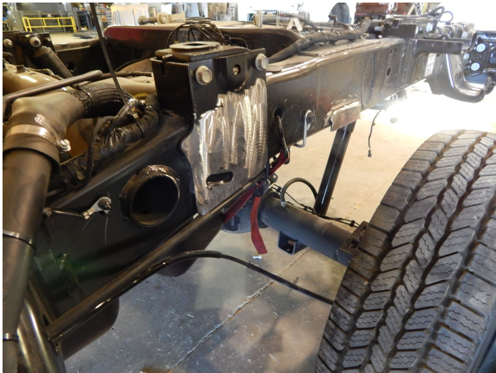
Overload perch shown removed from the frame.
