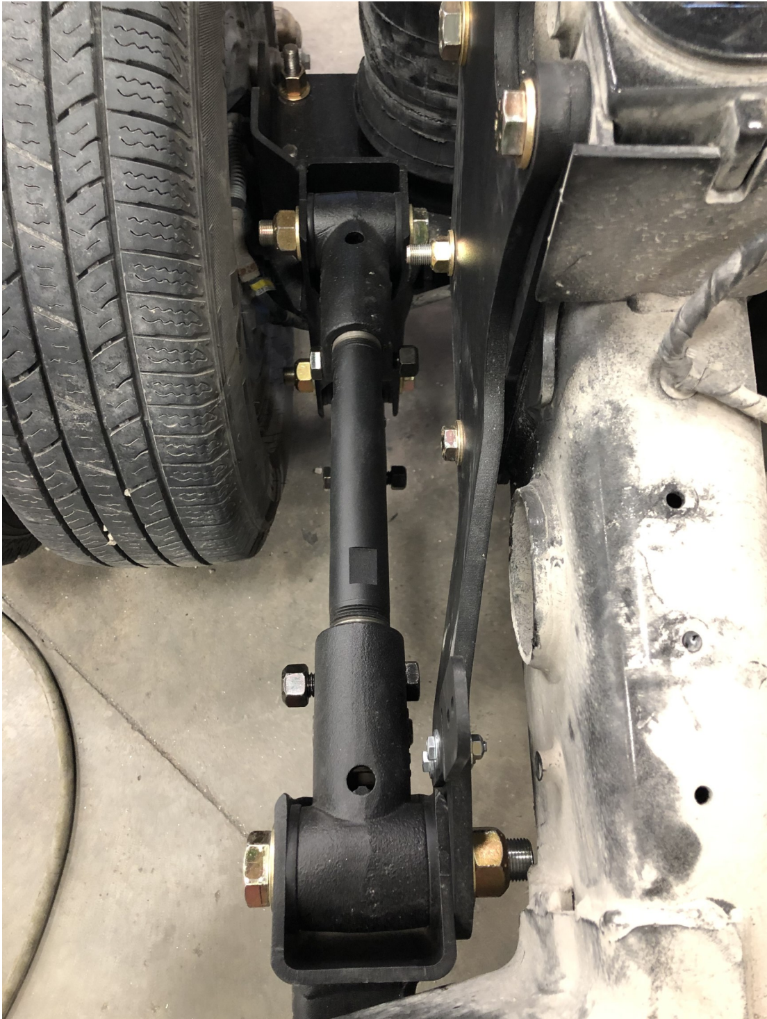
Trailing arms shown installed into forward mount and lower air bag mount
