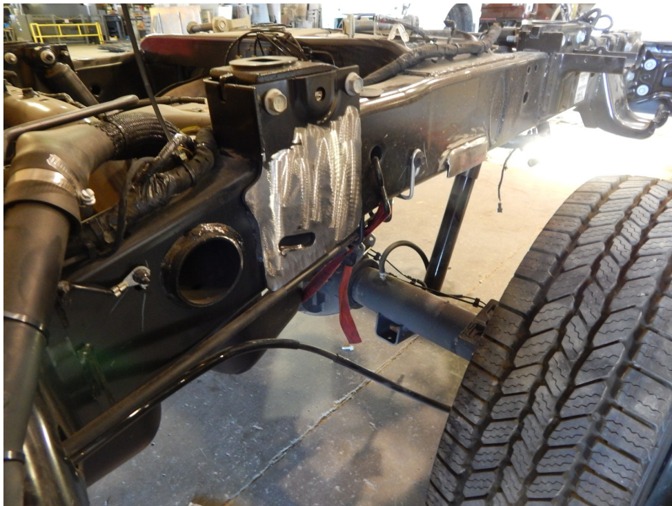
Overload perch shown removed from the frame.
