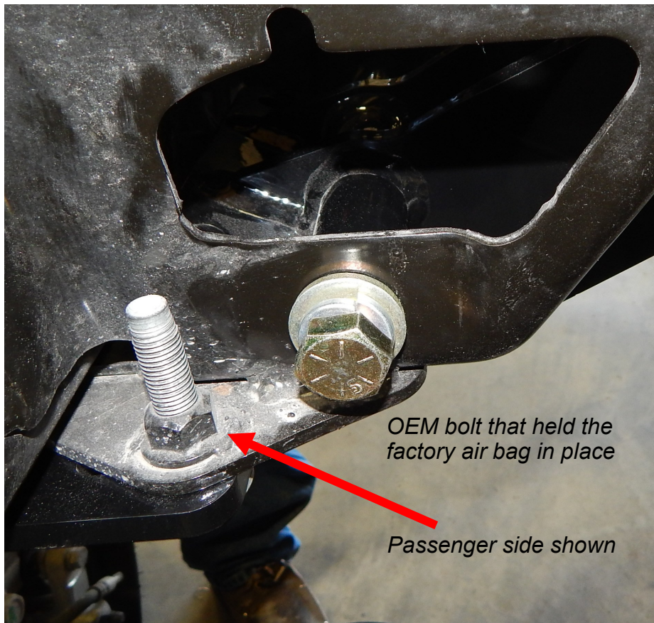
Panhard bar bolt plate replaces OEM bolt plate (passenger side)
