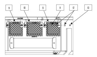
Bolt the lower screen (16) into the center section, using the supplied ¼" hardware (10, 11, & 12).
