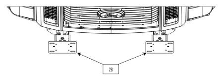
**6**: Use the studs of the bumper mount bolting tabs (3) to position the bumper on the frame brackets (26) Use washer (28) and nut (29) to fasten the bumper to the mount.
