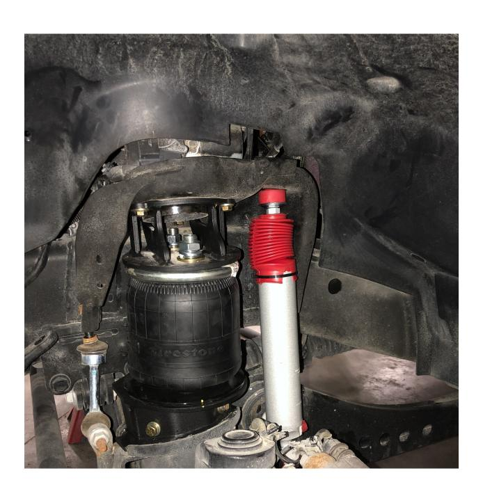
9. Plumbing of the air bags. (If you are not running height control valves or electronic sensors, go ahead and install the plastic inner liner now.
