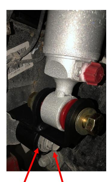
Use the OEM bolt to fasten the lower shock relocation bracket in place. Torque to 75 ft/lbs.
