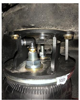
5. Now that the air bags and brackets are installed, locate the shocks (Part#80118-99042) and lower shock mounts (part#10004766DS and 10004760PS). Turn the dial on the bottom of the shock to setting 3. Setting 3 and 4 are where the ride quality is the best.
