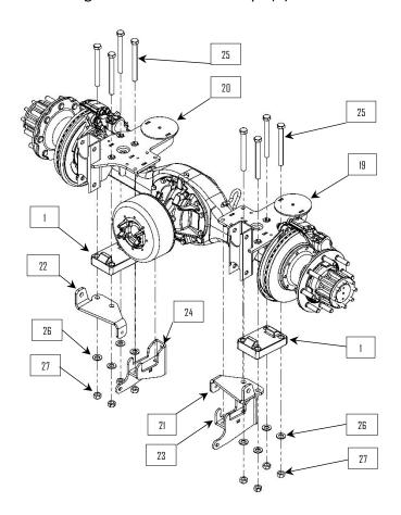
10: Bolt the panhard bar crossmember (28) to the lower bag plates (19 & 20) using 1/2" hardware (15, 18, & 29). Use 5/8" hardware (8, 9, & 30) to fasten lower axle clamps (23 & 24) to the axle. Align the holes on the lower shock ear plates (21 & 22) with the other components. Do not tighten hardware yet.
