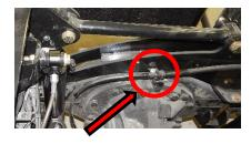
**29:** On the passenger side cut off the factory brake line bracket after the first hole and fasten it to the forward carriage bolt (17).
