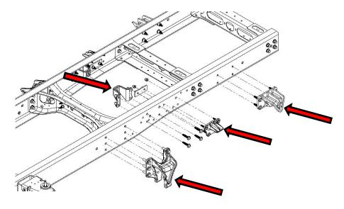
**13**: To remove the huckbolts split the nut using a cutoff wheel or an air chisel.
