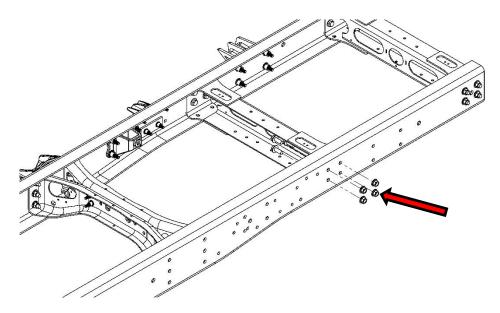
**16:** Proceed to *step 1* of the *Kit Installation* section of these instructions and install the Kelderman side plate onto the now bare frame rail.
