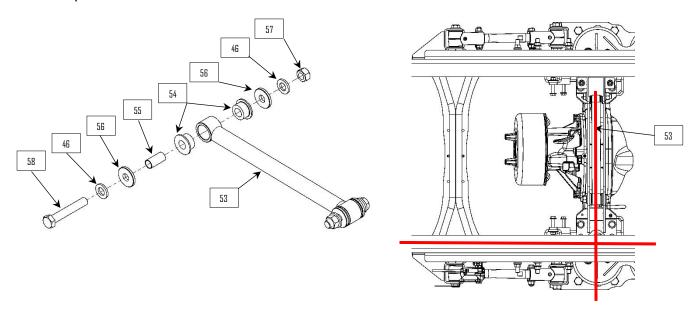
**23:** Grease sway bar bushings (59) and install onto sway bar (60). Install the d-rings (61) over the bushings (59) and fasten to the lower axle clamps (23 & 24) using 3/8" hardware (50, 62, & 63). **NOTE:** Install sway bar with the arms angled up and the center angled down.
