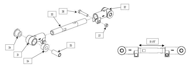
**12:** Use 7/8" hardware (38, 39, & 40) to install the lower trailing arm assemblies into the lower bag plates (19 or 20). Do not tighten hardware.
