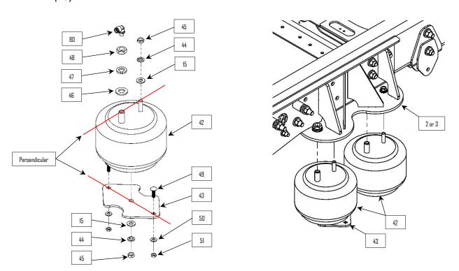
**16:** Bolt the air bags (42) to the side plate (2 or 3) using 1/2" hardware (15, 44, & 45) and 3/4" hardware (46, 47, & 48). **NOTE:** The air bag and plate assembly from step 15 goes toward the front of the truck.
