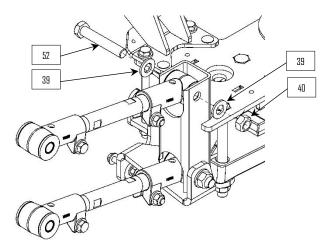
**19:** Bolt the upper and lower trailing arm assembly into the side plate (2 or 3) using 7/8" hardware (38, 39, & 40). **Torque:** 7/8"-14 trailing arm bolts should be torqued to 300ft-lb.
