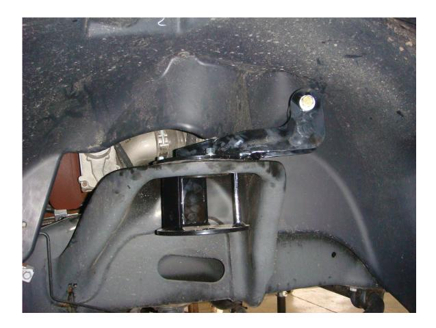
6. Locate the 5323 Firestone air bag. Locate the lower air bag/lower shock mount. Fasten the air bag to the bottom mount with the  $1/2 \ge 3 1/2$ " bolt and lock washer. Before torqueing the bolt, drop the assembly into place and jack up the axle to get the orientation of the top studs of the air bag with the top air bag mount. Once the bag location is determined, torque the  $1/2 \ge 3 1/2$ " bolt to 35 ft./lbs.
