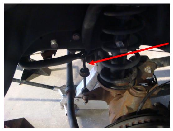
4. Remove the factory shocks. There is one bolt on the bottom of the axle and a mounting bracket on top of the spring bucket. Remove the three nuts that hold the upper shock mount. Keep the lower bolt and nut as it will be used to fasten the lower air bag mount in place.
