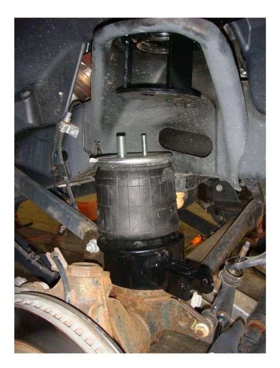
7. Once you have the air bag tightened to the lower bag mount, drop the air bag and lower bag mount into place on top of the axle. Locate the original 14 mm lower shock mount and nut. Wiggle the mounting bracket in place so the holes line up and fasten in place, torqueing the 14 mm bolt to 95 ft./lbs.
