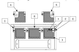
Place the lower screen (16) into the bumper and fasten in place with flat washer (12) hex bolt (11) and nut (13).
