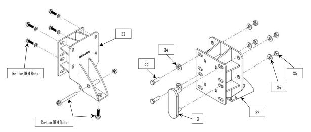
**11**: Install the bumper frame brackets *(32)*. Use OEM hardware from steps 7 & 8 to bolt the brackets to the frame horns.
