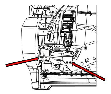
**3**: To access the grille first remove the black plastic panel in front of the radiator.
