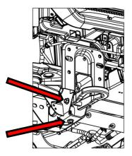
**9:** If equipped remove the parking sensors from the stock bumper. Spread the ears on the sensor bezel and push the sensor thru the back of the bumper. NOTE: Keep track of each sensors location.
