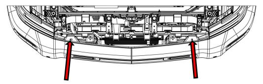
**6**: Remove the two bolts, one per side, located just inside and above each tow hook. The bumper can now be removed from the truck.
