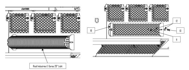
Bolt the end caps onto the center section using the supplied hardware. Repositioning may be required after bumper is installed onto truck. NOTE: While positioning use masking tape to protect painted surfaces that come into contact.
