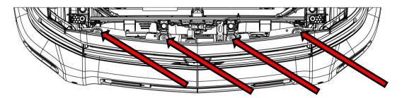
**5**: With the bumper supported remove the two bolts located on either side of the grille opening.
