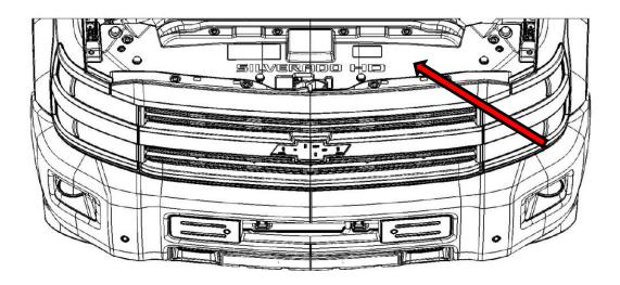
**4**: Remove the four screws that run across the top of the grille. The bottom of the grille is held in with clips. Pull outward at each clip location until it releases. The grille can now be removed.
