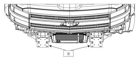
12: Use the studs of the bumper mount bolting tabs (3) to position the bumper on the frame brackets (32). Use washer (34) and nut (35) to fasten the bumper to the mount.
