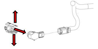
**10**: Depress the tabs on the sensor bezel and push it thru the front of bumper.
