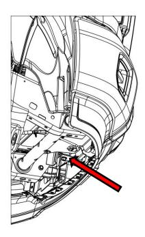
7: Remove the eight bolts that hold the bumper brackets to the frame horns. **NOTE:** These bolts will be reused for install.
