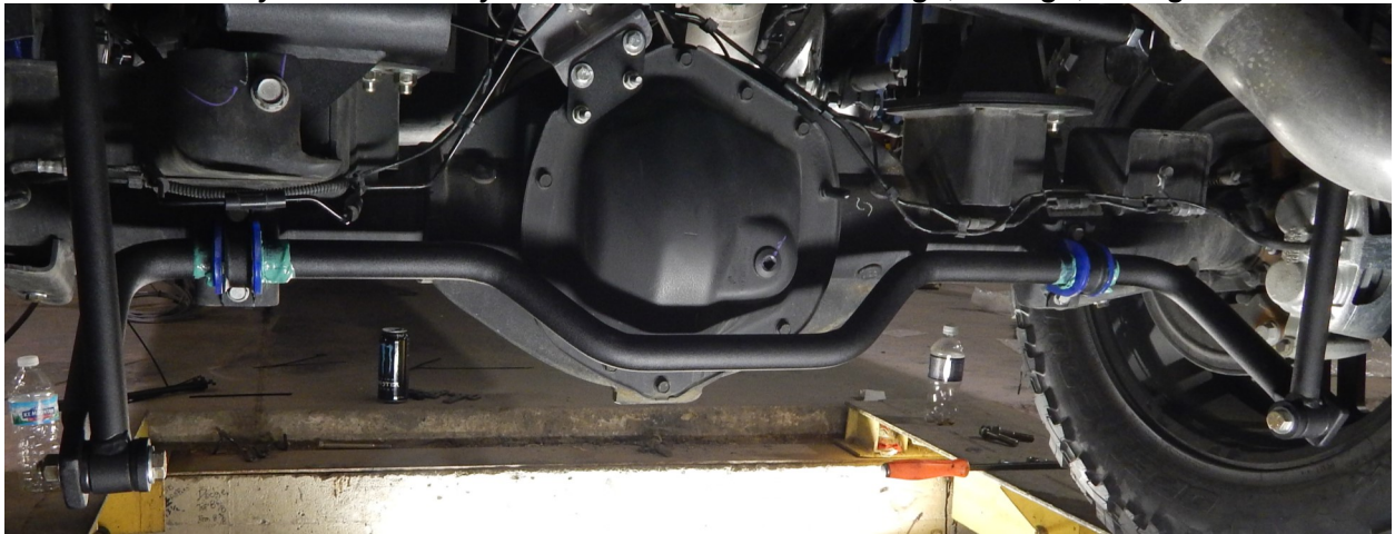
Rear sway bar assembly shown installed w/ bushings, d-rings, and grease
