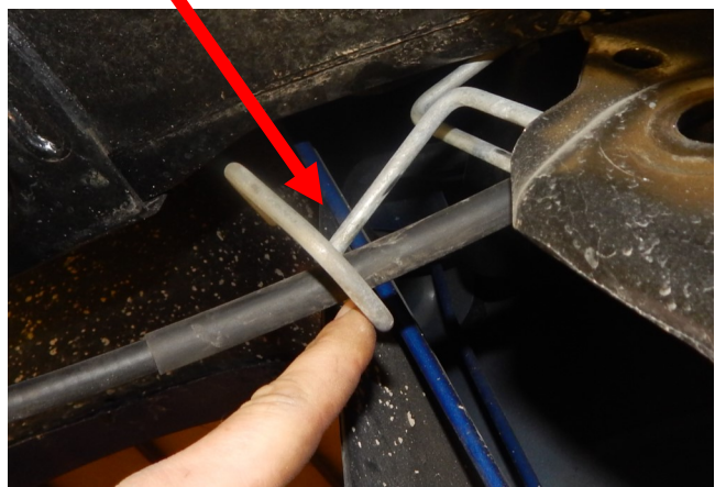
Remove drivers side e-brake cable from this loop
