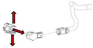
**6**: Depress the tabs on the sensor bezel and push it thru the front of bumper.
