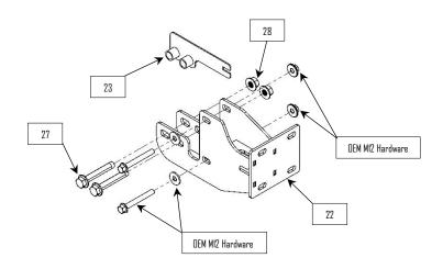
7: Insert the anti-crush bracket (23) into the frame horn. Re-use the OEM hardware removed in *step four* to bolt thru bumper bracket (21 & 22) and the frame horn. NOTE: Some trucks may already have factory anti-crush bushings located where the crash protector was installed. These trucks do not require the installation of anti-crush bracket (23).
