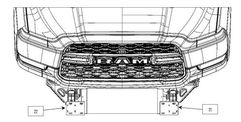
8: Install bumper bracket (22) on the passenger side and bumper bracket (21) on the driver side.
