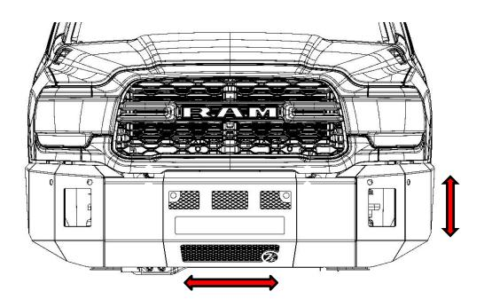
**11:** On trucks equipped with an intercooler install the air duct (29) using the hardware removed in *step three*. The air duct (29) will slide up behind the installed bumper.
