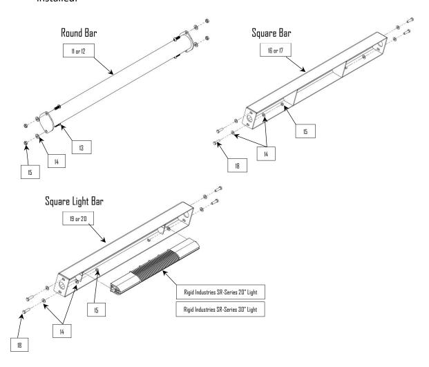
**8:** If optioned install lights into the crossbar using the hardware supplied with the light. **NOTE:** The light mounting ears will deform and draw up to the light as they are tightened.
