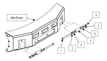
2: NOTE: On bumpers equipped with large winches the winch must be unbolted and slid over to access the tow hook bolts (1). Winches may be bolted thru the face of the bumper as well as thru the winch plate. On trucks equipped with parking sensors use care when moving the winch so as not to cause damage. Do not bolt the winch back in yet.
