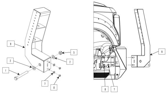
**6**: Repeat this process to install the grille guard horn (9 or 10) on the other side of the bumper. Tow hooks (4) and rubber washers (3) will not be reused.
