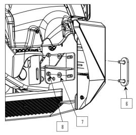
**5**: Insert the grille guard horn (9 or 10) into the pocket and bolt thru the frame bracket. The crossbar mounting holes should face the center of the truck. Reinstall the 7/8" tow hook bolt (1). Do not tighten down hardware; some movement in the grille guard horn will be required when installing the crossbars.
