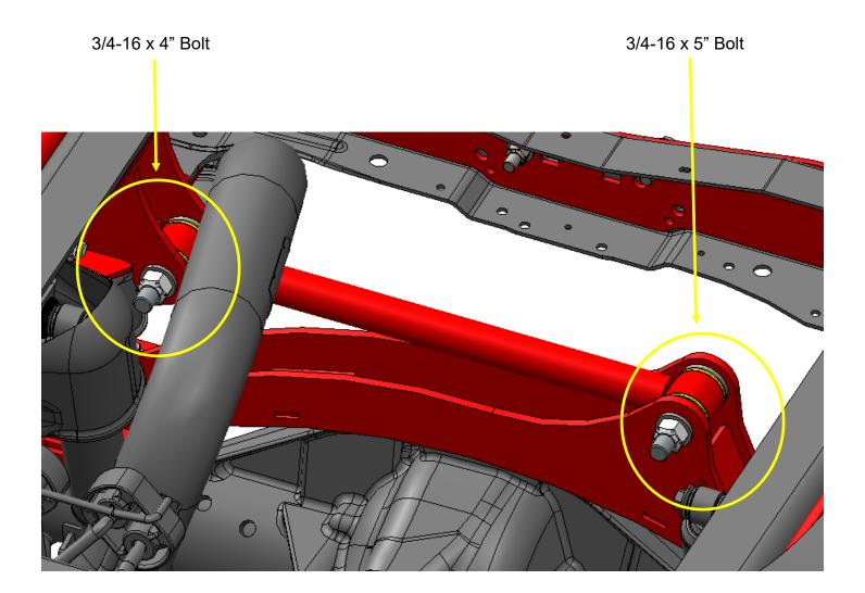
11. Locate the rear sway bar & Bushing Kit (#1139-190KLD). It fastens to the original OEM mounts with the factory bolts and D-ring. Use the new bushings provided. Use Loctite on the factory bolts.
