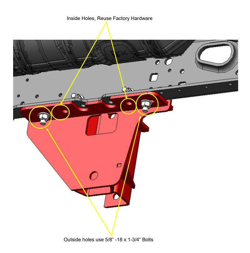
3. Locate Upper Pan Hard Bar Mount (#10015044). The upper PHB mount utilizes the bolts on the passenger side plate. Place inside the frame and tighten down.
