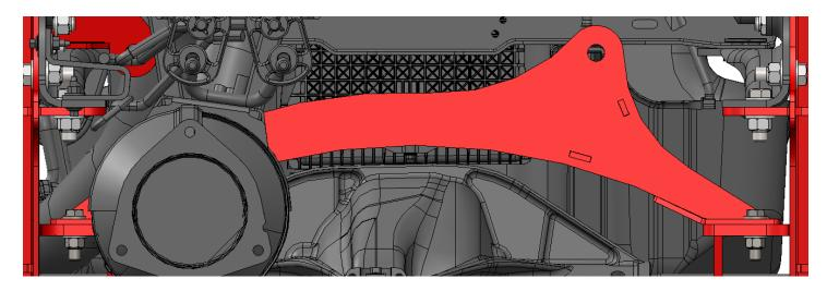
7. Locate Brake line relocation bracket (#10015222). Remove axle breather hose and fitting from axle. Place brake line relocation bracket over axle breather hole and reattach breather hose. Next angle factory brake bracket upwards and attach to relocation bracket with a 1/2"-20 x 1" bolt and nut. Ensure the brake hoses are pushed towards the outside of the vehicle (driver side).
