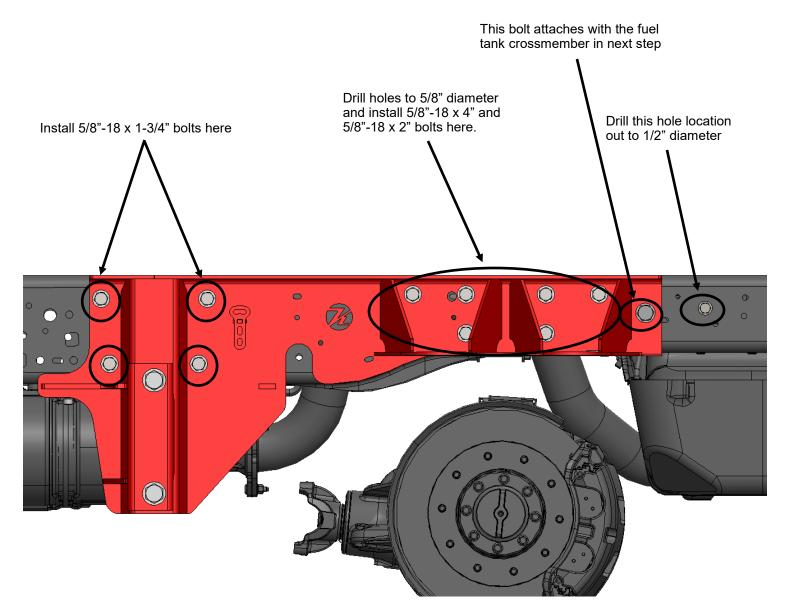
On bottom of side plates, use (2) 5/8"-18 x 1-3/4" bolts on the outside, slotted holes. Reuse the factory bolts for the inside holes.
