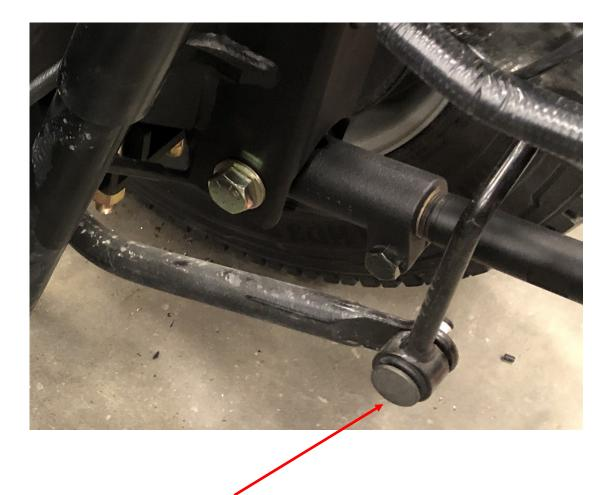
Attach sway bar to factory OEM end links
