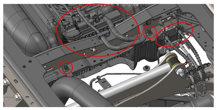
Install corner brace weldments (10015051 & 10015053) with (2) 3/4"-16 x 2-1/2", (2) 3/4"-16 x 2" bolts and (4) 1/2"-20 x 2" bolts.
