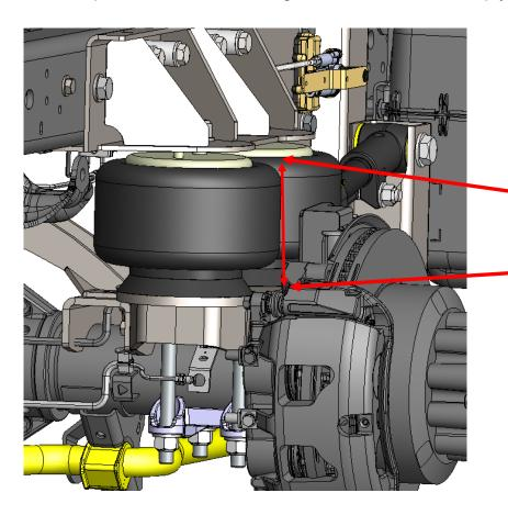
Set the air bags so there is **7-7/16**" between the mounting brackets that hold the air bags in place
