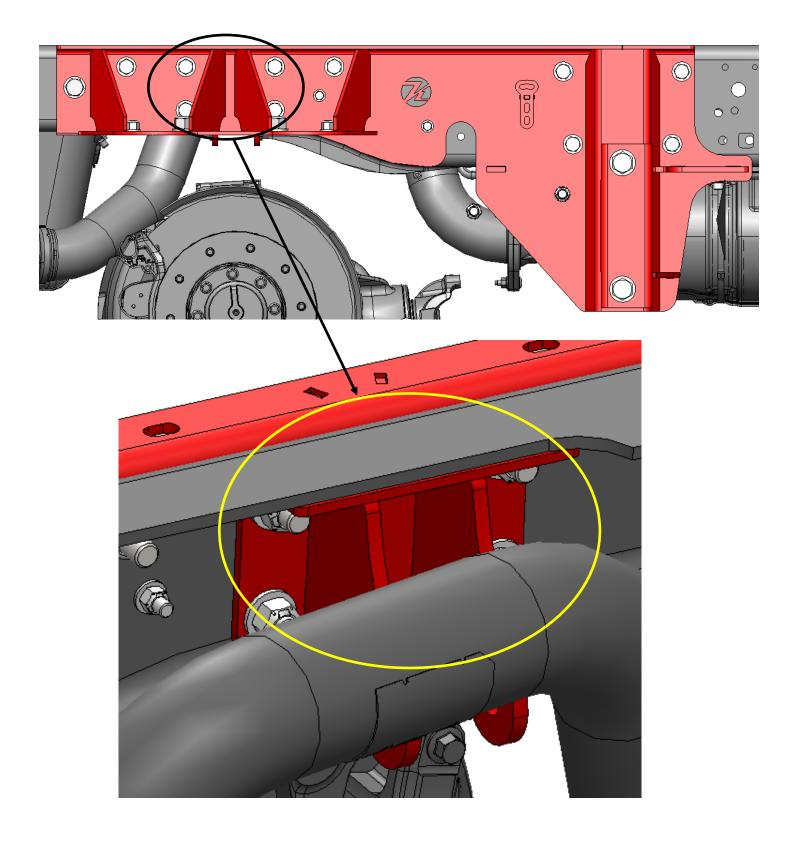
4. Locate the (3) piece fuel tank cross member parts (#10015070, 10015051 & 10015053). The kit mounts inside the frame rails and across the back side of the factory cross member in front of the fuel tank. To assemble backing plate (#10015070), loosen fuel tank strap bolts and let the tank drop a bit. A jack will be necessary to hold the weight of the fuel tank. Also may be necessary to disconnect fuels line that may be in the way. Disconnect brake line bracket and move to the side.
