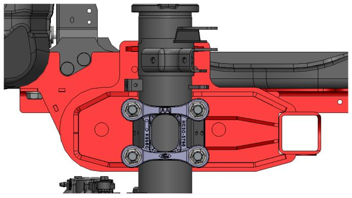
6. Locate Crossmember (#10015038) and attach to DS/PS Lower Bag Mounts with (4) 1/2"-20 x 2" bolts. Make sure the upper part of crossmember is opposite the upper PHB mount "Drivers Side".
