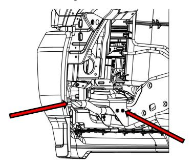
**3**: With the bumper supported remove the two bolts located just under the grille on either side of the black plastic bumper insert. **NOTE:** The grille must be removed to gain access to these bolts.
