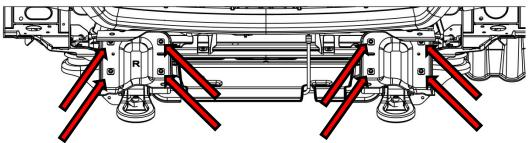
8: Remove the four bolts that hold the tow hooks. NOTE: These bolts will be reused for install.
