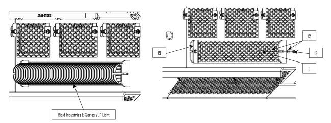
Bolt the end caps onto the center section using the supplied hardware. Repositioning may be required after bumper is installed onto truck. NOTE: While
