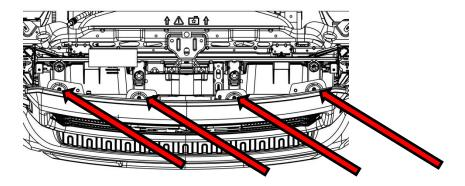
**6**: Remove the two bolts, one per side, located just inside and above each tow hook. The bumper can now be removed from the truck.
