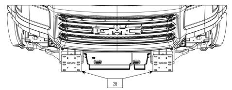
12: Use the studs of the bumper mount bolting tabs (3) to position the bumper on the frame brackets (28). Use washer (30) and nut (31) to fasten the bumper to the mount.
