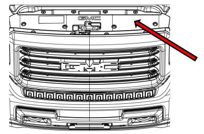
**5**: Remove the four screws that run across the top of the grille. The bottom of the grille is held in with clips. Pull outward at each clip location until it releases. The grille can now be removed.
