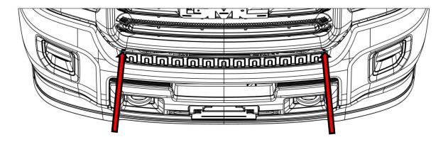
**4**: To access the grille first remove the black plastic panel in front of the radiator.
