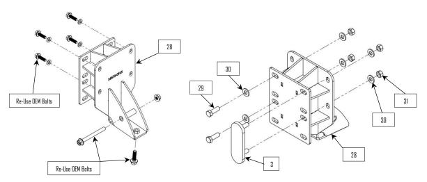
**11**: Install the bumper frame brackets *(28)*. Use OEM hardware from steps 7 & 8 to bolt the brackets to the frame horns.
