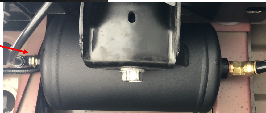
Slight angle keeps fitting from hitting crossmember and pinching the wiring harness shown.
