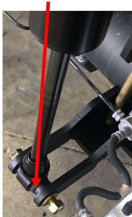
Lower shock spacer goes towards the tire side
