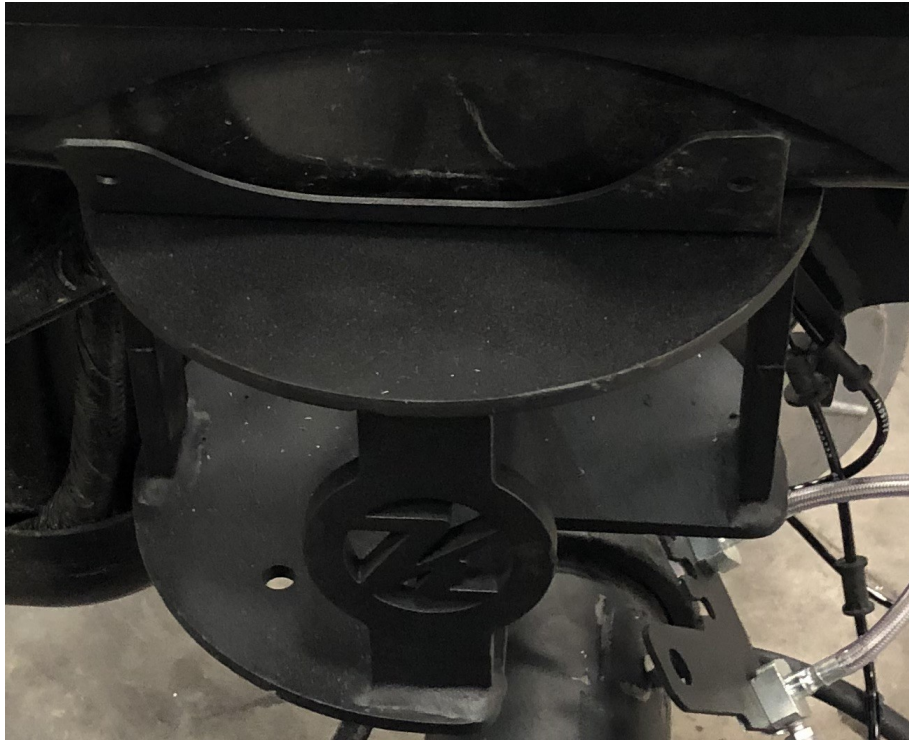
Crossmember connects to the upper bag mounts with the 1/2" x 1-3/4" bolts
