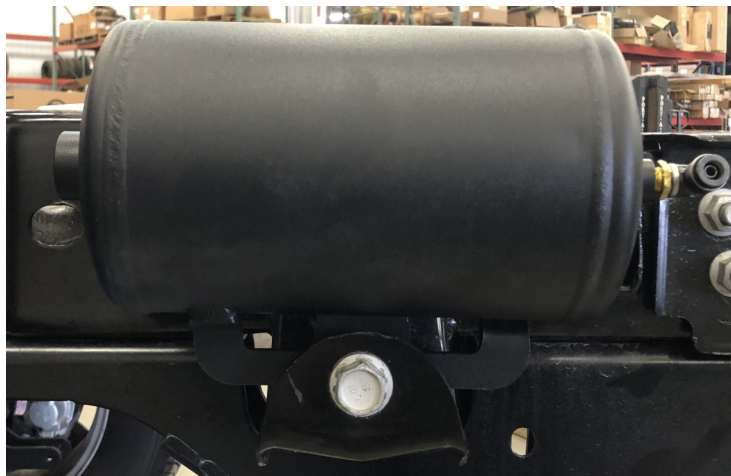
Slight angle keeps fitting from hitting crossmember and pinching the wiring harness shown.
