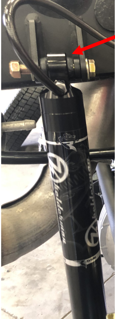
Upper spacer goes on front side of the shock
