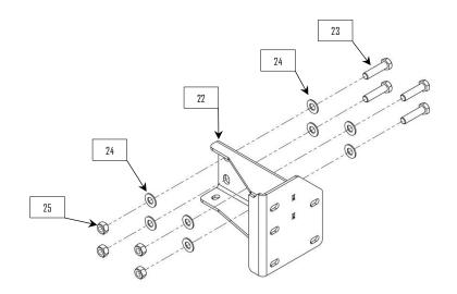
5: Install bumper frame brackets (21 & 22). Bolt the frame brackets thru the frame and leaf spring hanger using the 5/8" bolts (23) flat washers (24) and lock nuts (25). Reuse the bolts from Step 3 to fasten thru the frame bottom flange.
