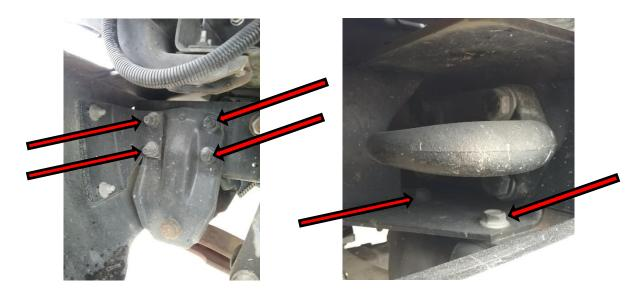
**4**: Remove the factory tow hooks and bumper bracket, they will not be re-used.
