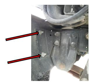
3: Lift the frame of the truck enough to take the weight off the front leaf spring. Leave the front tires on the ground to support the axle. Place a floor jack under the front leaf spring hanger. Remove the two bolts from the bottom of the bracket (these will be reused) and the four bolts from the side of the bracket. Use the floor jack to keep the hanger bracket in place. WARNING: Do not remove bolts while spring is loaded.
