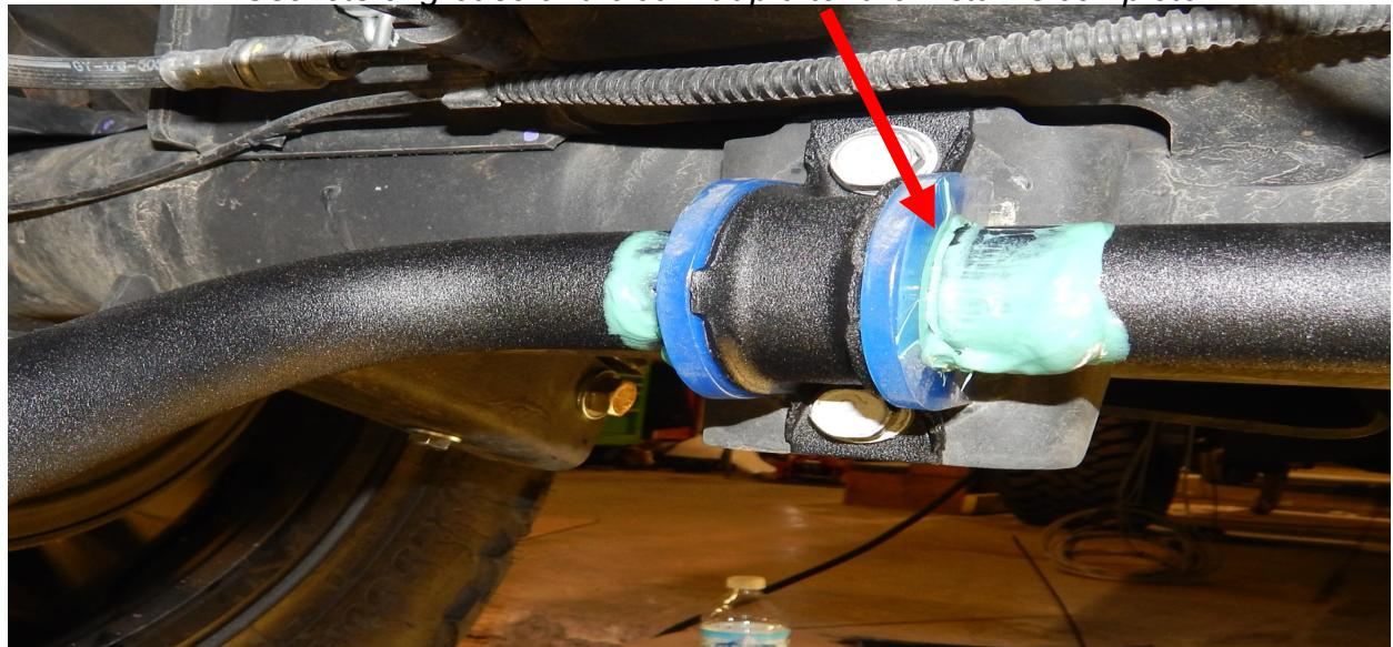
15.) Locate the sway bar end links (Part # XXXX) and the upper end link mount adapters (Part # 19161). The upper end link adapters fasten to the factory end link mounts with the 1/2 x 3" bolts and the 3/8 x 1 1/4" bolts. Fasten the bottom of the end link to the sway bar with the 1/2 x 3" bolt. Make sure to use the large flat washer on the outside of the end link (against the poly bushing). Torque the 1/2" bolt 85 ft./lbs. and the 3/8" to 45 ft./lbs.
