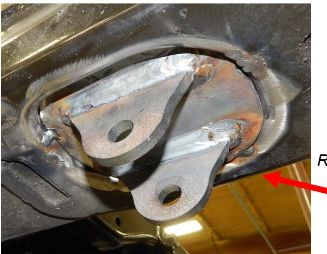
13.) With the shock mounts are installed, locate the shocks (Part # 10095 Raptor) and install. Use the xx bolts on top and OEM 14mm bolts on the bottom to fasten into place. Torque the bolts to 95 ft./lbs.
