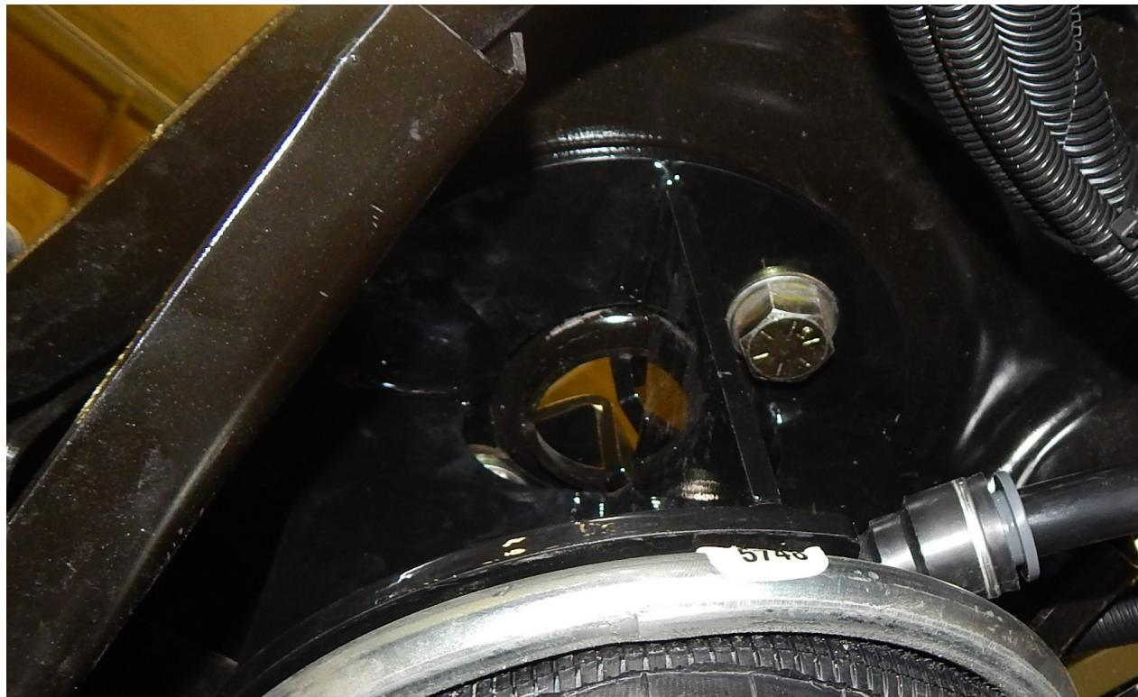
4.) Locate the brake line relocation bracket (Part # 19046). Remove the two nuts off the mounting studs and slide the relocation bracket over the studs. Fasten with the factory nuts. Torque to 20 ft./lbs. Fasten the brake line bracket to the relocation bracket with the 1/4 x 1" bolts. Torque to 25 ft./lbs. Examine the brake lines along the axle. Once the install is complete, make sure the brake lines are not rubbing on anything. *New brake lines are not required for this kit.*
