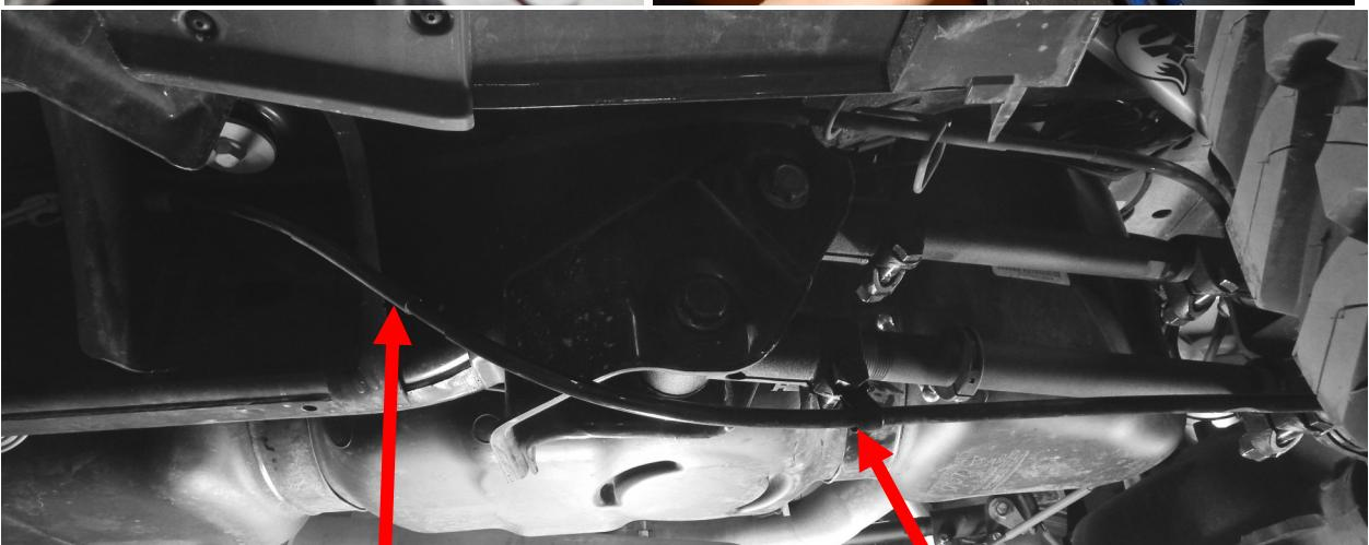
*Brake cable now drops down below the rear mount that it originally was routed through*
