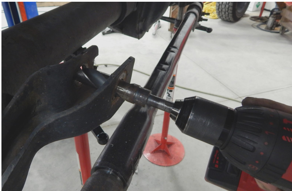
The lower pan hard bar mount on the axle is removed for the 9-10" kit.
