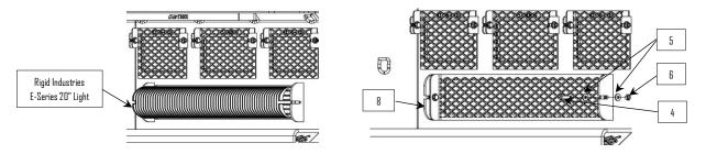
Bolt the end caps (9 & 10) onto the center section using the supplied hardware (11, 12, & 13). Re-positioning may be required after bumper is installed onto truck. **NOTE**: While positioning use masking tape to protect painted surfaces that come into contact.
