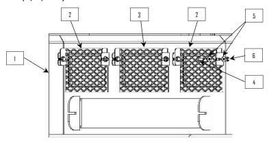
Bolt the lower screen (7) into the center section, using the supplied 1/4" hardware (4, 5, & 6).
