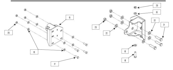
**4:** Use 5/8" hardware (21, 22, & 23) to bolt the bumper brackets (15 & 16) into the frame horns. Use 1/2" hardware (18, 19, & 20) to fasten thru the bottom flange.
