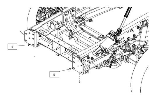
**5**: Install bumper bracket (16) on the passenger side and bumper bracket (15) on the driver side.
