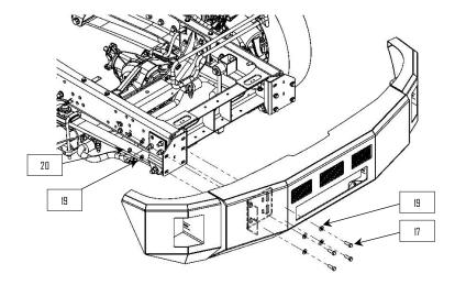
**1:** Align the bumper on the truck and tighten the mounting hardware. Slowly open the hood and check that it clears the bumper. NOTE: The end caps can be re-adjusted at this point if required.
