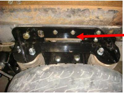
Drill this hole **CAUTION! Make** sure to not drill into any fuel or brake lines
