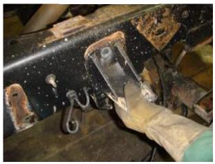
4. The best way to remove the riveted pads is to use a torch to cut the rivet heads off. Make sure that there are no fuel lines, brake lines, or wiring that can be damaged while cutting the rivets off.
