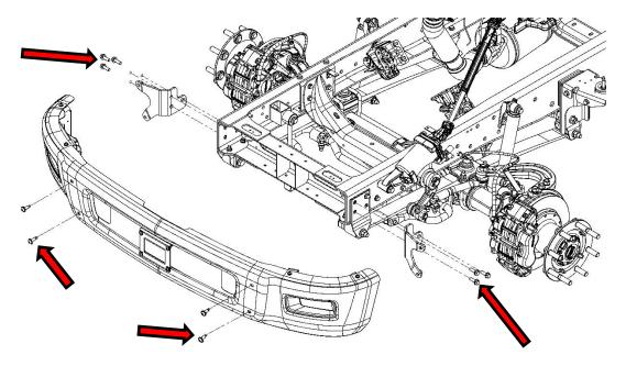
**3**: Remove the front two bolts from the bottom flange.
