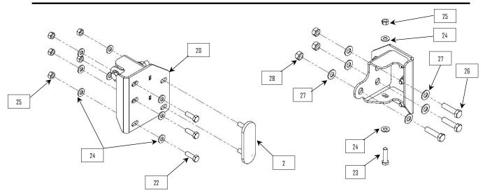
**4**: Use 5/8" hardware (26, 27, & 28) to bolt the bumper brackets (20 & 21) into the frame horns. Use 1/2" hardware (23, 24, & 25) to fasten thru the bottom flange.
