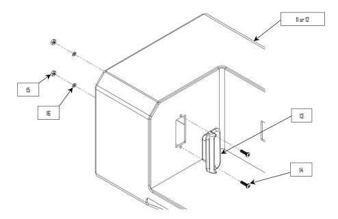
If optioned, install the reverse lights into the center section.
