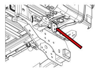
**4**: Remove the two bolts from each side that fasten the bumper bracket to the tow hitch. Save these as they will be re-used later when installing the new brackets. The bumper brackets can now be removed.
