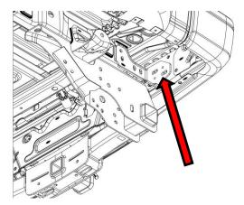
**3**: Remove the two bolts from each side that fasten the bumper bracket to the frame. Save these as they will be re-used later when installing the new brackets.
