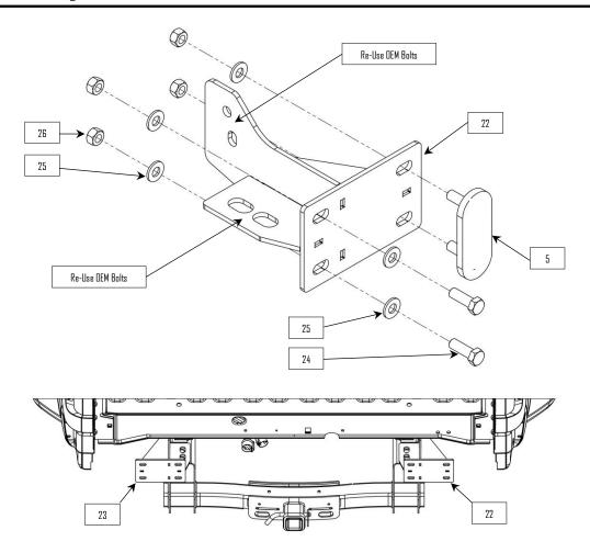
8: Install the bumper frame brackets (22 & 23). Re-use the hardware removed in steps four and five.
