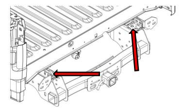
**5**: If equipped remove the parking sensors from the stock bumper **NOTE**: Keep track of location. Spread the ears on the sensor bezel and push the sensor thru the back of the bumper.
