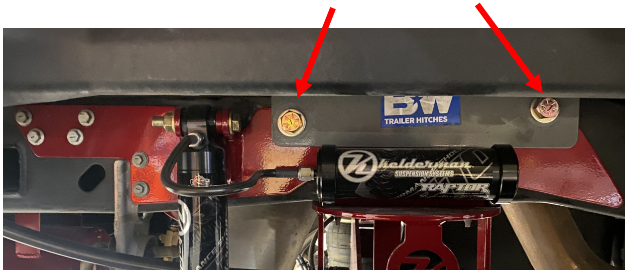
Passenger side shown with shock installed
