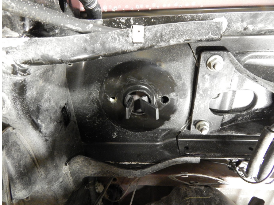
Upper Air Bag Mount Shown Installed
