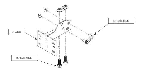
7: Install the bumper frame brackets (22 & 23). Re-use the hardware removed in steps four and five.
