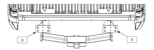
8: Use the studs of the bumper mount bolting tabs (5) to position the bumper on the frame brackets (22 & 23). Use washer (25) and nut (26) to fasten the bumper to the mount.
