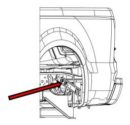
**3**: Remove the four rear bolts that fasten the receiver hitch to the frame. Save these as they will be re-used later when installing the new brackets. **NOTE:** Complete removal of the hitch is not required.
