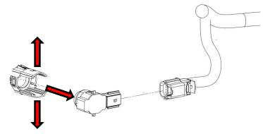
**5**: Depress the tabs on the sensor bezel and push it thru the front of bumper.
