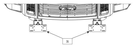
7: Use the studs of the bumper mount bolting tabs (3) to position the bumper on the frame brackets (26) Use washer (28) and nut (29) to fasten the bumper to the mount.
