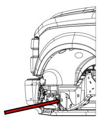
3: With the bumper supported remove the four bolts located on either side of the two tow hooks. The bumper can now be removed.
