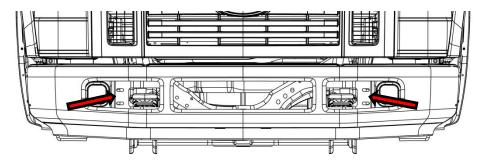
4: Remove the six bolts that fasten the tow hooks to the frame. These will be reused during install.
