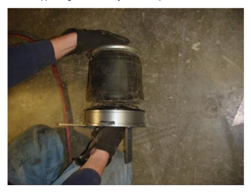
6. Set the Lower Air Bag Mounts on top of the axle They fasten to the axle with the 3/8" x 1-1/2", bolts (and Spacer Part# 50789), 3/8" x 1" bolt and and 1/2" x 1-1/2" bolts. The 3/8" x 1" and 1/2" x1-1/2" use the tab nuts, being that there is no way to get a wrench on the nuts.
