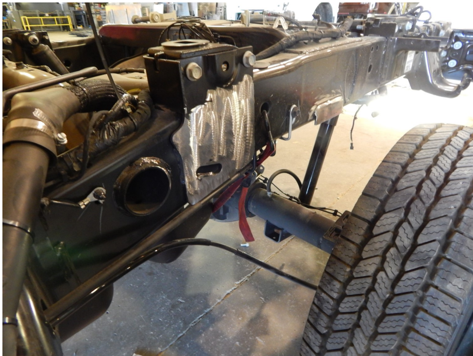
Overload perch shown removed from the frame.
