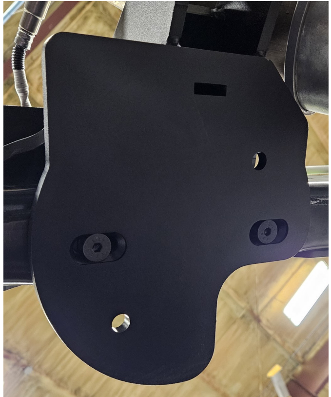
Drivers Side shown with M10 bolts installed.
