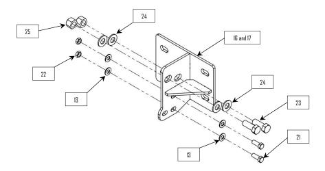
**4:** Use 9/16" bolts (23) to install the bumper frame brackets (16 & 17). Drill out the two lower holes to accept the 3/8" bolts (21).
