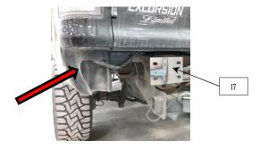
**6:** Use ½" bolts (18) to position the bumper on the frame brackets (16 & 17). Use washer (19) and nut (20) to fasten the bumper to the mount.
