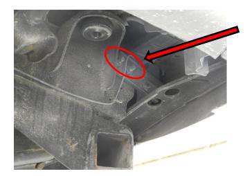
**3:** Remove the trailer light plug bracket from the hitch.
