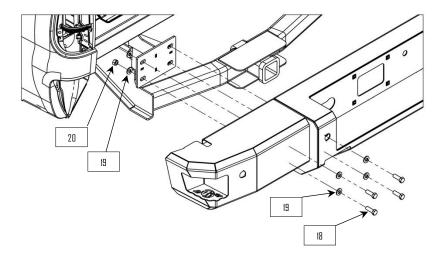
**7:** Align the bumper on the truck and tighten the mounting hardware. **NOTE:** The frame brackets may need to be re-adjusted to get the depth correct.
