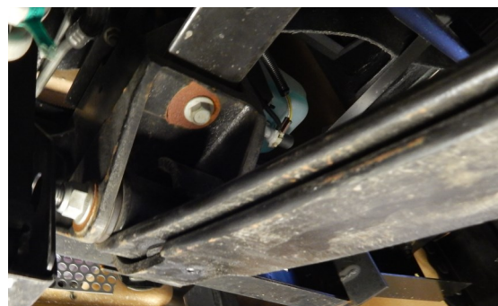
Front leaf spring installed in factory perch
