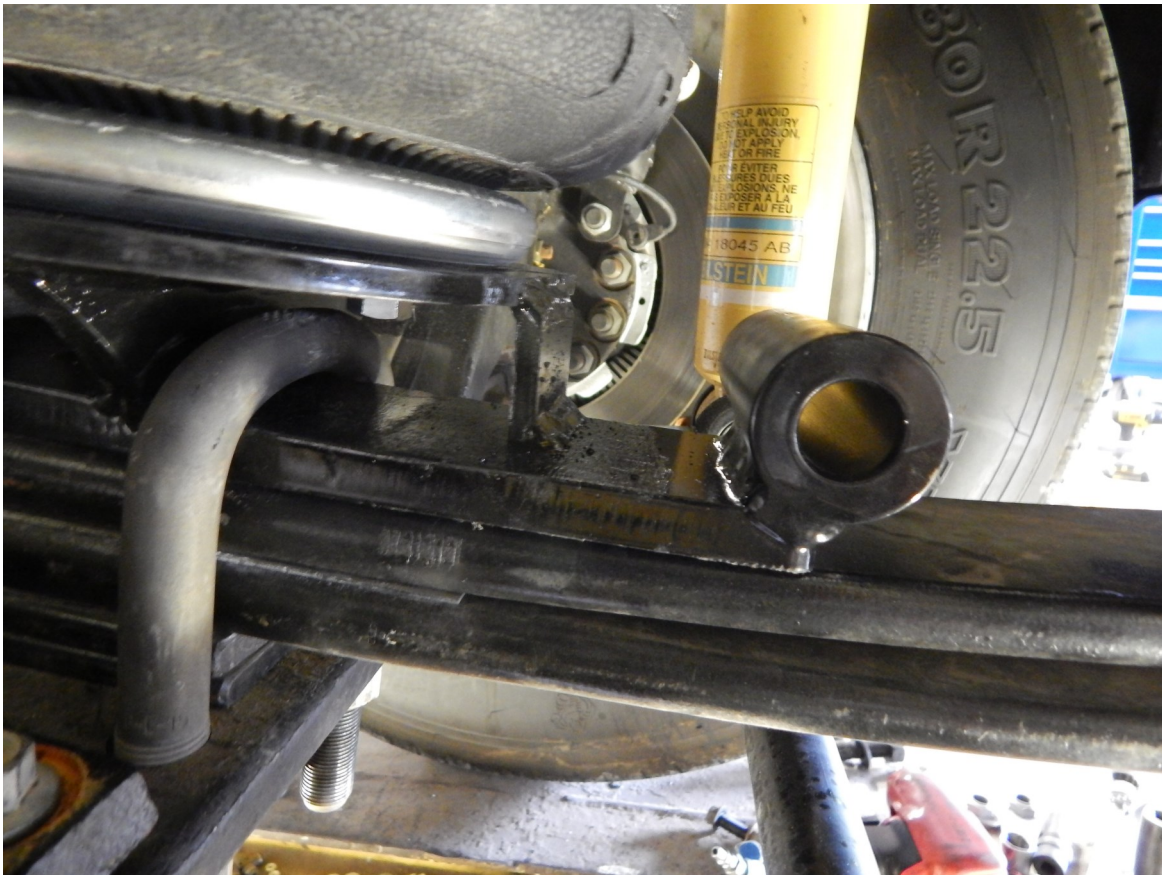
Front leaf spring installed in factory perch
