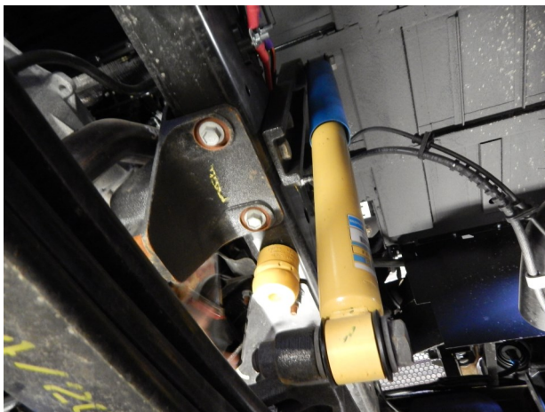
Remove the socks, sway bar and rubber bump stop
