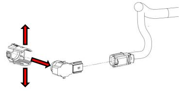
7: Depress the tabs on the sensor bezel and push it thru the front of bumper.
