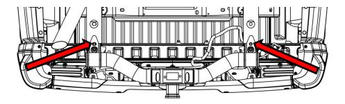
4: With the bumper supported remove the remaining three bolts from each side that fasten the bumper bracket to the frame. The bumper can now be removed.
