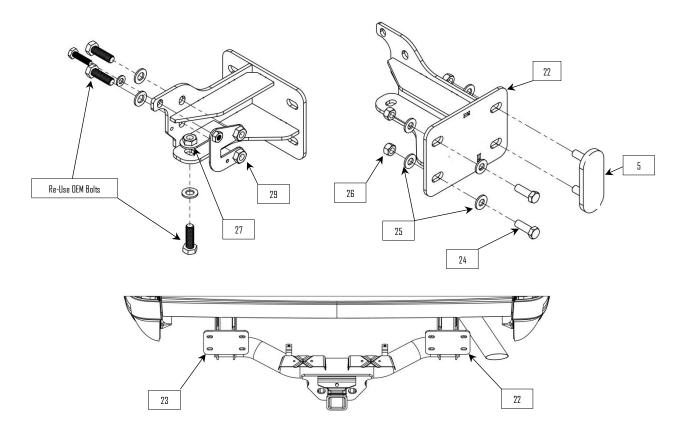
**9:** Install the bumper frame brackets (22 & 23). Re-use the hardware removed in steps four and five.
