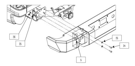
**10**: Use the studs of the bumper mount bolting tabs (5) to position the bumper on the frame brackets (22 & 23). Use washer (25) and nut (26) to fasten the bumper to the mount.
