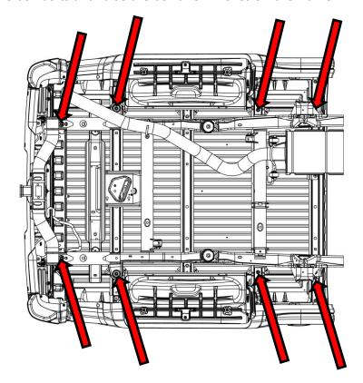
**3:** Remove the two bolts from the bottom flange of each bumper bracket.
