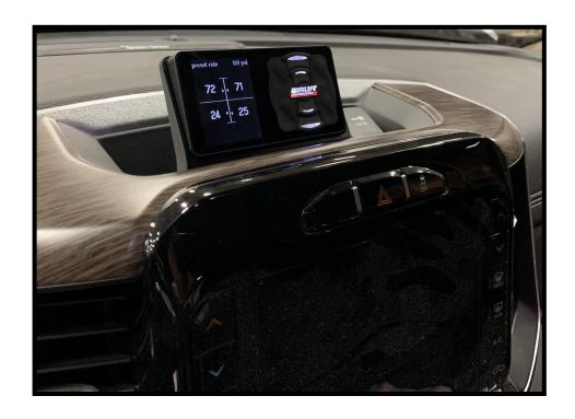
1. Install the provided USB extensions cable (*figure a*), then install the chord shim ensuring the shim is flush with the back of the screen (*figure b and c*). Next, remove the (2) screws that hold the touchpad in place (*figure d*). Remove the touchpad (*figure e*) and rotate to the correct position: screen to the left and "airlift" logo right-side up (*figure f*). Reinstall the screws (<u>take care not to overtighten</u>).
