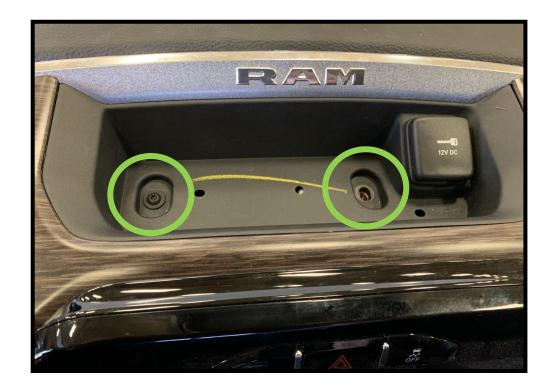
2. Securely grab the center dash unit and pull towards the rear of the vehicle to remove.
