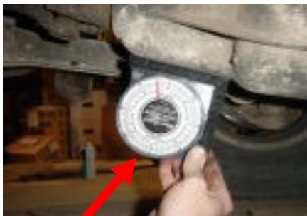
Use an angle finder to get pinion angle recorded off the bottom of the axle
