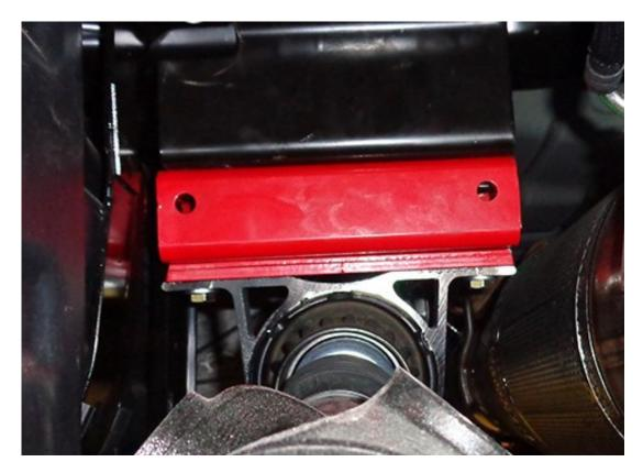
14. Locate the shocks. The part number will vary depend on what brand and what style was purchased. The upper end should slide over the oem stud. On the bottom, use either the factory bolts or the supplied 1/2" bolts to install, depending if the shocks have 1/2" or 14 mm spacers. You may have to use a washer or two as spacers on each side of the shock if they are narrower than your OEM shocks. Torque these bolts to 85 ft/lbs.
