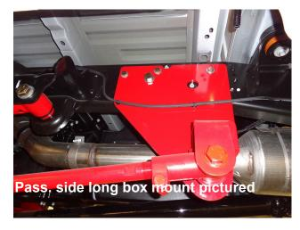
Notch the fuel tank cover for clearance for the forward trailing arm side mount (long box, drivers side). On short box trucks its just as easy
