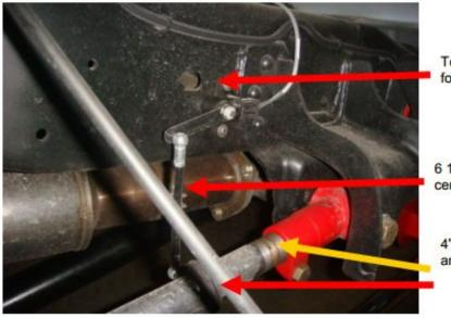
Top of sensor is 5/8" forward of the hole
