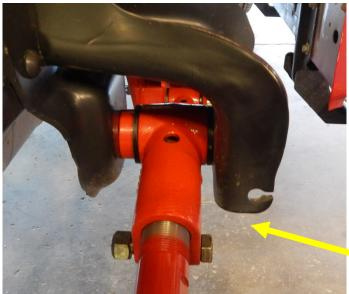
ing arm mount. Presetting the trailing arms at those distances should allow the final adjustment to be easier. If the arms get more than 1/4" off in length (top left compared to top right and bottom left compared to bottom right) they will bind when adjusting. Use the supplied flat washer on each side of the 7/8 bolt. Tighten these bolts to 275 lb/ft.
