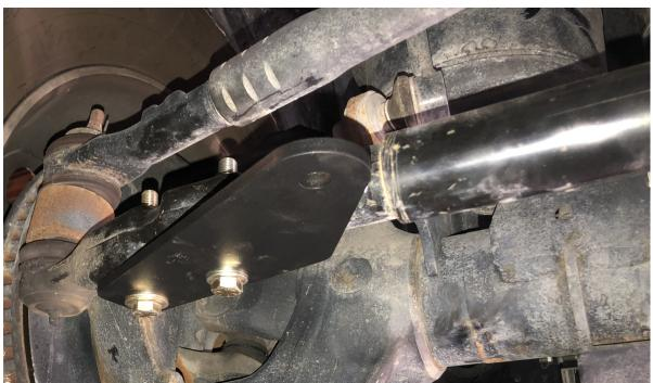
9. Locate drivers side shock mounting plate (10012101) & attach to drivers side steering link. Locate (3) factory M12 bolts and hardware. Rotate the tie rod tube and tube clamp so that the mounting plate is parallel with the stabilizer bracket.
