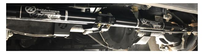
**Note:** Make sure shocks are level with steering link before torquing down bolts.
