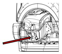
**3**: With the bumper supported remove the eight bolts located on either side of the two tow hooks. The bumper can now be removed.
