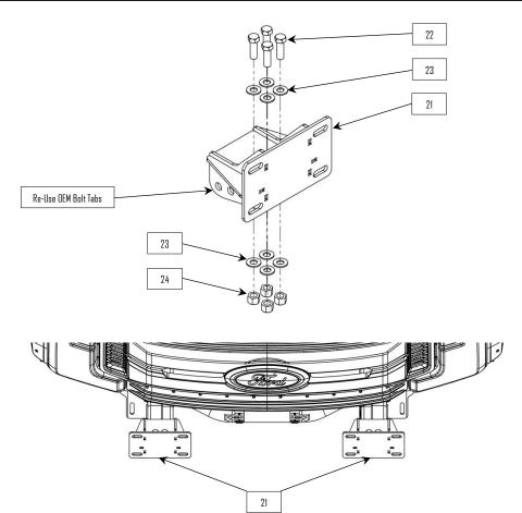
**5**: Install the bumper frame brackets (21). Use the provided 9/16" bolts (22) and nuts (24) to bolt thru the top of the frame. Re-use the bolt tabs from step 4 to bolt thru the sides of the frame.
