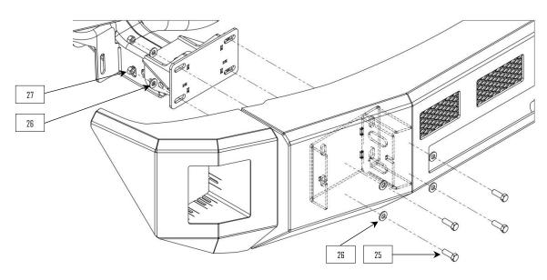
Bravo Series Front Bumper Installation Manual – 2017 Ford Super Duty
