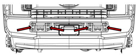
4: Remove the eight bolts that fasten the upper bumper brackets and tow hooks to the frame. Remove the four bolt tabs that fasten the lower bumper brackets to the frame. The four bolt tabs will be reused during installation.
