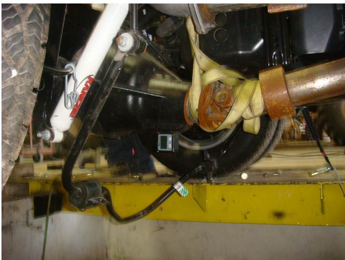
Sway bar dropped from the axle. Passenger side shock attached at the bottom mount only. The strap is used to keep the pinion angle somewhat close to the correct setting.
