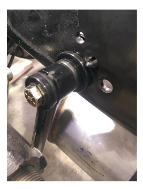
1. The Ram 4500/5500 chassis cabs have a different exhaust than the 84" and longer chassis. This requires a different end link set up than shown in the instructions provided in the kit. The 60" kit uses longer endlinks and they attach to the side of the frame. Use the pictures below to see which hole to use. You will want to drill the hole out to 1/2". Make sure to use the machined washer on the outside of the bushing. Torque the 1/2" bolts to 85 ft/lbs.
