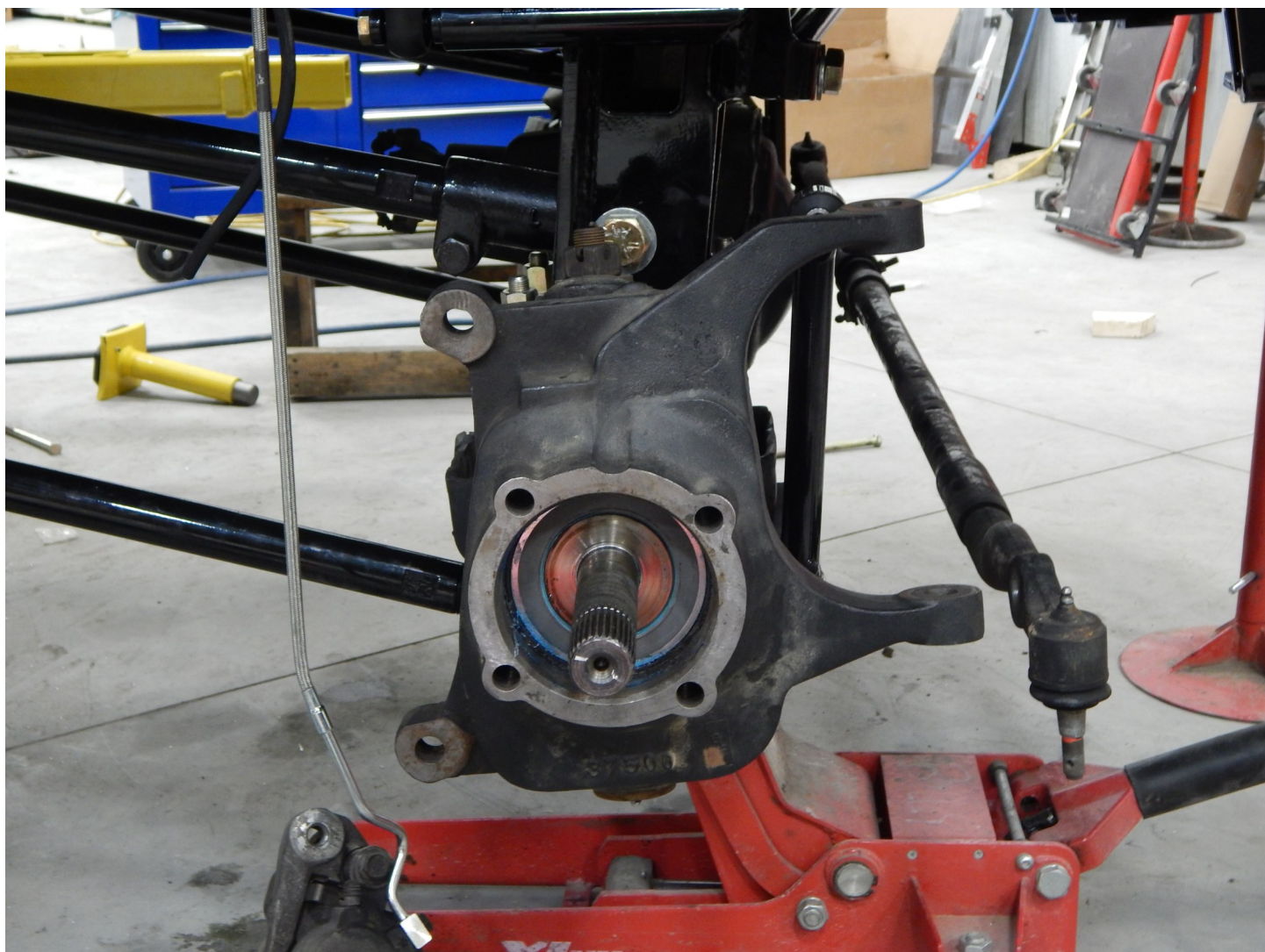
Cross over steering knuckle installed
