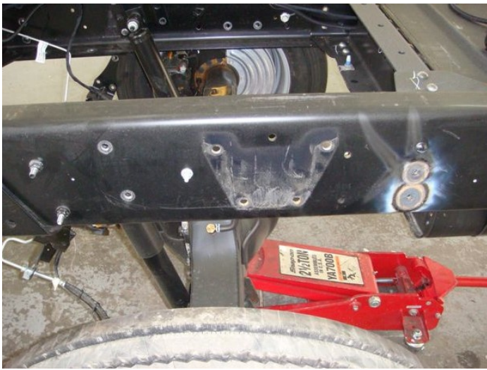
Place jack under axle to keep from rotating.
