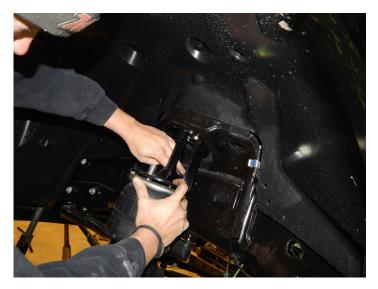
**NOTE:** The passenger side upper spring bucket has a gusset welded on from the factory. The drivers side does not have this bracket. A weld in bracket is supplied for the drivers side (Part # 18436). Once you have the air bag installed, wrap up the air bag and mounts and weld the gusset in place. Make sure not to put the gusset to close to the air bag or it will rub on it. Once you have this mount welded in, paint it black to
