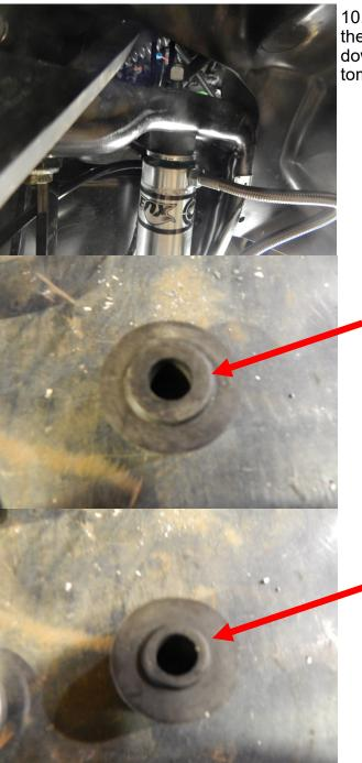
10. Place a bushing over the shock shaft so the large ring is down. Put the washer dish down. Thread on the lock nut until it bottoms out.
