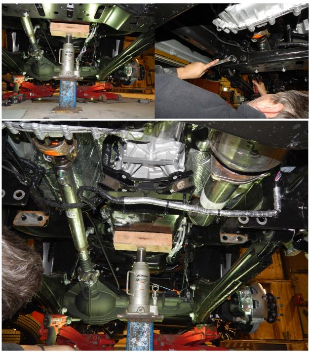
3. Locate the crossmember (part # 18291). It fastens into the factory cross member holes with the four 5/8 x 6 1/2" bolts. Use the M18x40 bolts to fasten the side of the cross member into the original control arm mounts. Torque these bolts to 150 ft./ lbs. Locate the three factory transmission nuts and fasten them to the crossmember. Torque to 40 ft./lbs.
