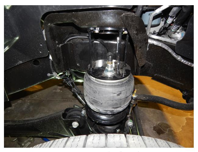
9. Locate the shocks and lower shock mounts (part # 18378). Fasten the lower end of the shock into the shock mount with the 9/16 x 5 1/2" bolt and slide the round end of the mount in the factory shock location on the axle. Torque this bolt to 125 ft./lbs. Locate the rubber bushings and steel cups. Place a cup (dish side up) on the shock and then slide a bushing (large ring up) over the shock and slide into the factory shock mount.
