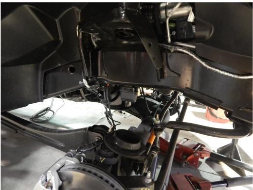
2. Place a jack under the transfer case. Remove the 3 nuts from the transmission mount where it fastens to the cross member. Remove the 4 bolts that hold the transmission cross member in place and remove the crossmember. Remove the 2 bolts that fasten the radius arms to the frame. Keep the nuts for the transmission mount, the other bolts will not be used.
