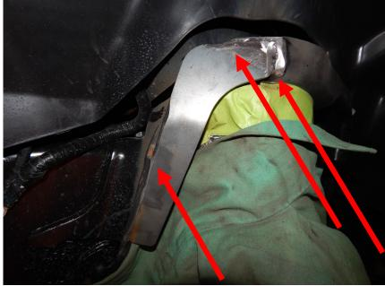
Weld the gusset into place to support the bucket.
