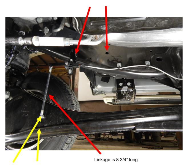
Center of ball stud to ridge on control arm 1 3/4" center of ball stud to trailing arm pivot bolt 27"
