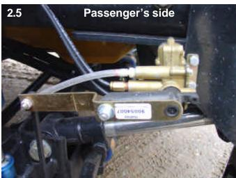
21. Locate the adjustable linkages that attach to the end of the height control valves. Use the 1/4" x 1 ½" bolt to fasten linkage to the end of the height control valve and to the hole by the shock mount on the lower bag plate. Adjust the linkage so the bags are 8" tall when inflated.
